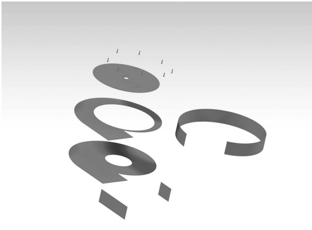
Figure 28: Exploded view of the impeller's casing. In this view all the individual flanges can be seen before welding together
