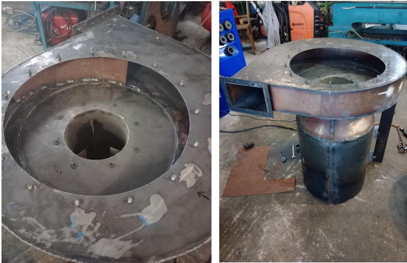
Figure 29: Result of manufacturing process of the impeller's casing.
