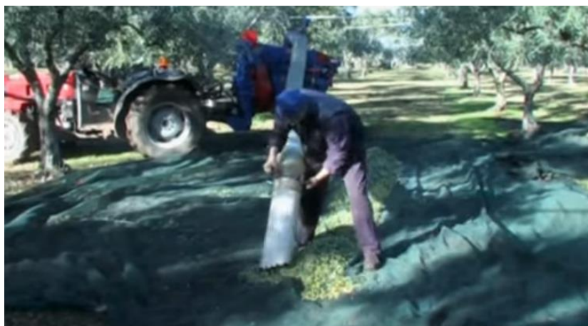
Figure 1: Aspirator device on the field gathering olive fruits. [Source: Youtube video - Agrioil aspiratore idraulico raccolta olive]
