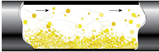
Figure 12: Mixed phase of conveying where the bottom section of the cross-sectional area of the pipe a bed of slowly moving particles is formed [Source: www.powderbulksolids.com ]
