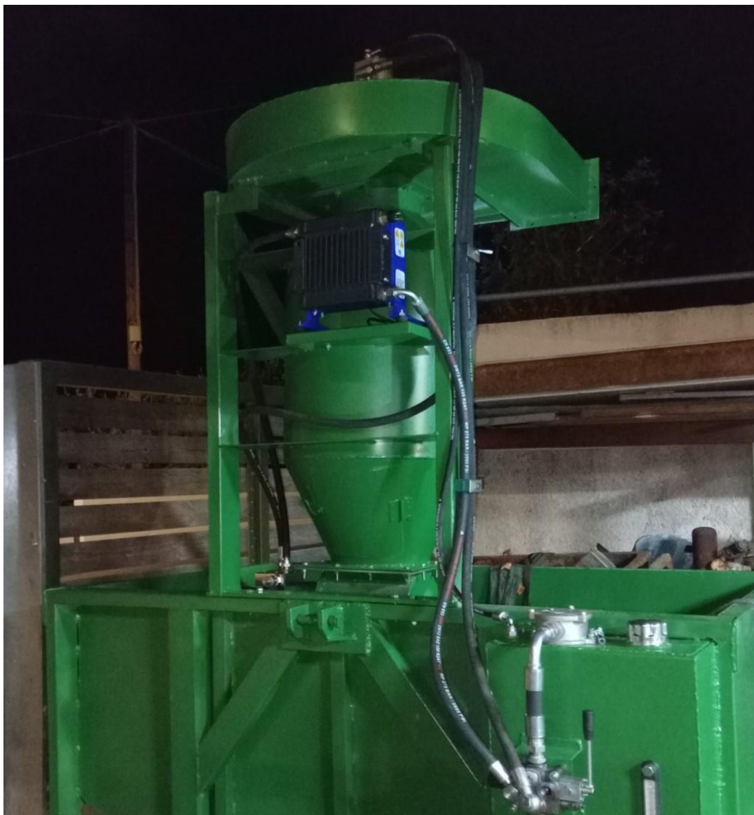
Figure 24: Aspirator device with cyclone. The assembly of the device includes the hydraulic system for the impellers rotation.
