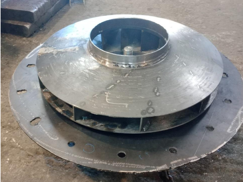
Figure 35: The fan is mounted to the shaft. Also, the shaft is supported to the bottom flange of the casing.
