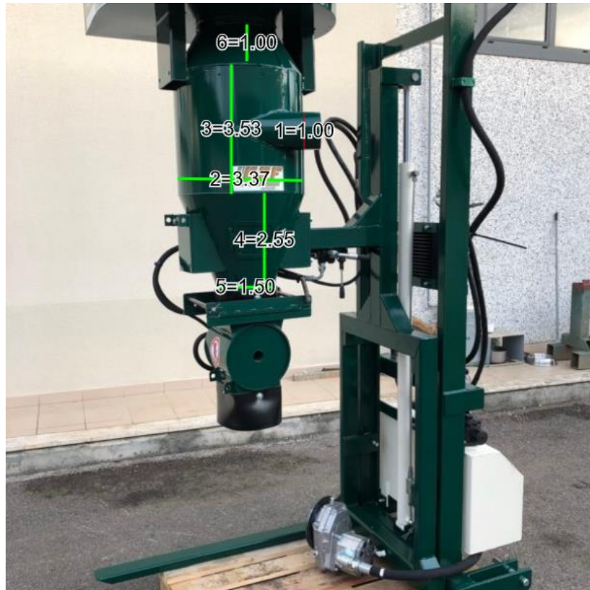
Figure 23: Pixel ratio of cyclone's parameters relative to the hose's inlet flange. [Source for image: "crfcostruzioni.it", source for image measurements: "https://eleif.net/photomeasure"]
