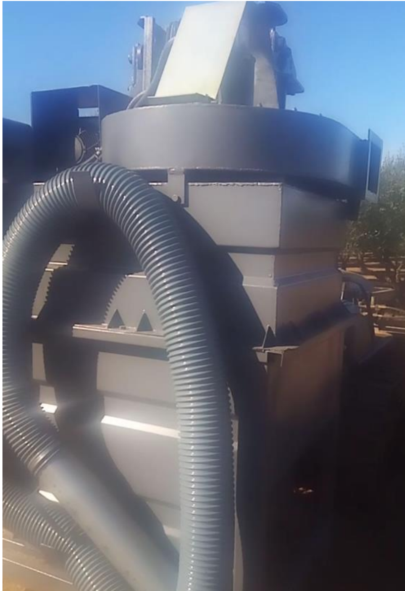
Figure 56: Box aspirator device completed assembly.
