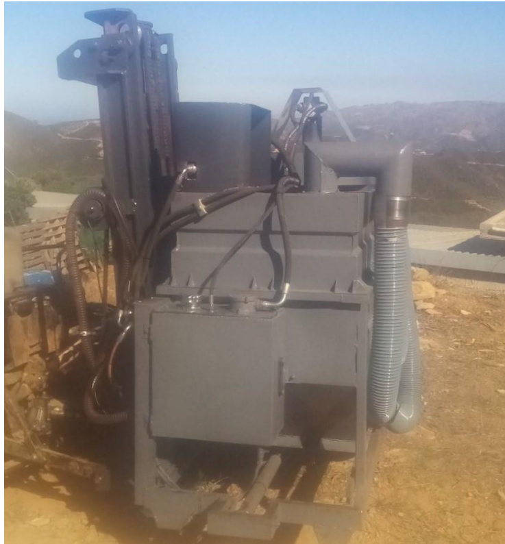
Figure 47 Aspirator device with rectangular box. The hydraulic system for the impeller's rotation is also visible.
