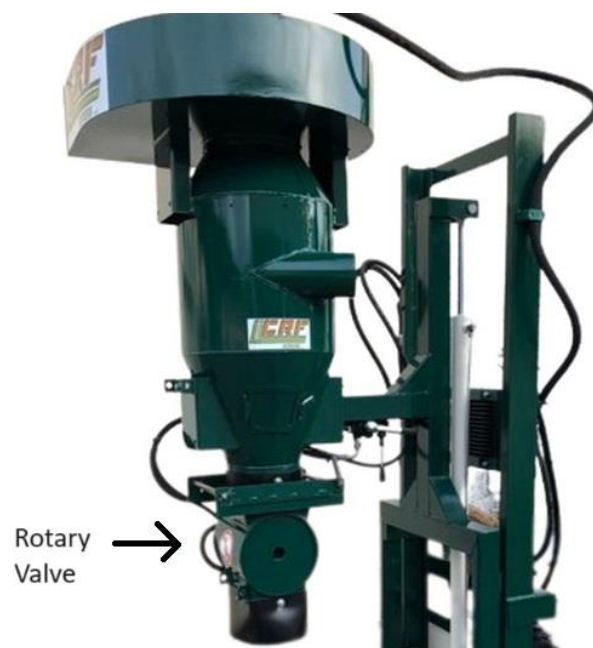
Figure 57: Rotary valve component, mounted at the bottom of the cyclone. The continuously rotating vanes inside the rotary valve casing unload the olive fruits at a constant rate. [Source for image: " crfcostruzioni.it "]
