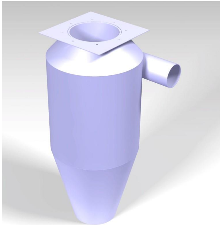
Figure 18: 3D model of cyclone designed in CAD software.
